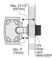
NOTE: Ensure compliance with the outside vent terminal location before cutting hole as both dimensions must be met.
